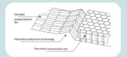
ThermHex honeycomb cores are made with a backing film of polypropylene as standard. This prevents the ingress of resin into the cells during processing, and therefore safeguards uniformity in the mechanical characteristics of the finished component. This also reduces the quantity of adhesive required to the minimum necessary. Polyester fleece layers on both sides are used to finish, achieving a surface for perfect bonding with the core.
