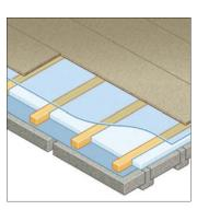
Caberfloor on battened floating floor
