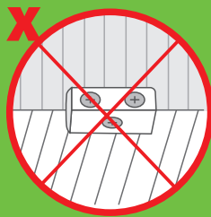
Incorrect fixed bracket
