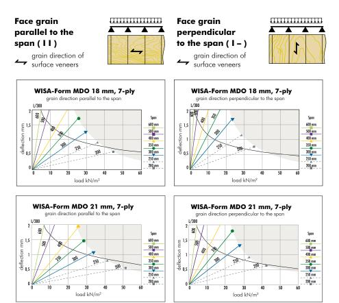
Moisture content 27 %, short term loading Partial safety factor for the material is 1.3. Partial safety factor for the loads is 1.2. Deflection limit L/300 of the span Support width is not taken into account in calculations
