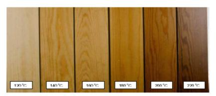
Figure 20-4. The colour of heat-treated pine. Treatment temperatures from 120 to 220°C at 20°C intervals. Treatment time (photo: VTT).
