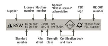
The chain of custody (COC) number demonstrates that the timber is from a legal and sustainable source. North American graded timber is accepted in Europe under BS EN 14081 and may be marked J&P (joist and plank grade) or NAMSR (North American machine stress-rated lumber).
