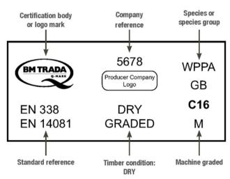
An additional visual assessment takes account of strengthreducing characteristics not automatically sensed by the machine.
