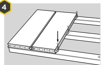
Take the next piece of deck and securely push into the Slim Clips. Now nip the screw to secure the Slim Clip against the board. **Do not over tighten**. Repeat steps 3 and 4 to cover the deck, using one Slim Clip and screw on every joist.
