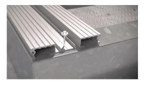
**NOTE:** Where boards are being fixed to a rigid substrate (for example a steel balcony) allowance must be made for thermal expansion by predrilling an 8mm hole in the base of the board at each fixing position, and leaving a min 3mm gap between board ends on runs in excess of .
