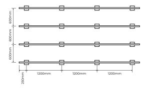
Set out a cleat foot at each point required using appropriate spacings along the length of the Boxrail<sup>™</sup>, usually 1200 - 1500 mm (refer to technical data sheets if unsure)
