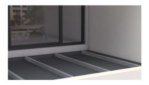
60 x 40mm **Boxrail<sup>™</sup>** or 50mm **Support Rail** – rails should be spaced at maximum 600mm apart with cleats at maximum 1200mm apart along the rail. Max overhang of joist beyond pedestal or cleat 250mm.
