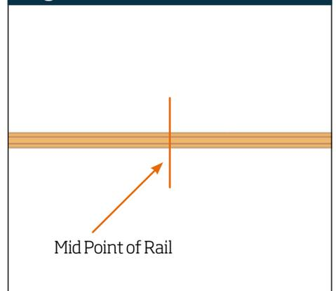
Fix the intermediate connectors to each end of the marked handrail. Offer the end of the handrail half way into the intermediate connector (**Fig.5**).
