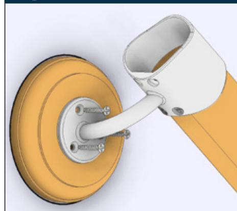
To fix rail for the bottom part of the stairs, offer the right hand end bracket onto the end of a handrail. Pilot drill through bracket screw holes using 3mm dia drill bit and secure using screws supplied (**Fig.13**).
