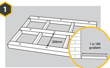
We recommend using a similarly fire rated subframe and allow for a gradual gradient of at least **1 in 100** (1%) that runs away from any adjoining buildings. Boards should run lengthways down this gradient to help water naturally disperse.
