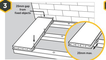
To secure the first board, use one Slim Clip and screw on every joist. Take a screw, place in the hole located in the Slim Clip and screw into the subframe. Make sure the boards do not overhang the joist at the edge by **more than 20mm** and a **20mm expansion gap** should be left between the wall or other fixed objects surrounding the deck.
