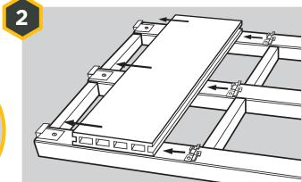
Place the first piece of decking on the subframe with the decking running perpendicular to the joists. The first piece of deck should be secured with starter clips. **Do not screw or nail through** *HD Deck 150® Fire*, use one Slim Clip and screw on every joist.
