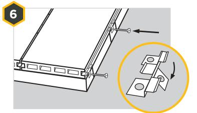
In order to fit the final board, bend the Slim Clip screw hole to a **90° angle** and fit over the edge of the subframe. Screw into place to secure boards. If necessary, you can trim the excess tabs off.
